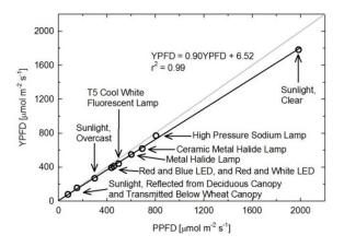
Correlation between photosynthetic photon flux density (PPFD) and yield photon flux density (YPFD) for multiple different radiation sources. YPFD is approximately 90 % of PPFD. Measurements were made with a spectroradiometer (Apogee Instruments model PS-200) and weighting factors shown in previous figure were used to calculate PPFD and YPFD.
