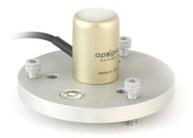
MQ-510 sensor attach to AL-100 leveling plate
