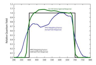
Radiation weighting factors for PPFD (black line, defined plant response to radiation), YPFD (blue line, measured plant response to radiation), and Apogee SQ-500 Series Quantum Sensors (green line, sensor sensitivity to different wavelengths of radiation).
