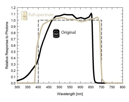
Mean spectral response measurements of six replicate Apogee SQ-100 (original) and SQ-500 (full-spectral) series quantum sensor. Spectral response measurements were made at 10 nm increments across a wavelength range of 300 to 800 nm in a monochromator with an attached electric light source. Measured spectral data from each quantum sensor were normalized by the measured spectral response of the monochromator/electric light combination, which was measured with a spectroradiometer.
